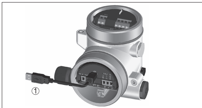
Fig. 29: Connecting the PC via USB to the Modbus electronics
