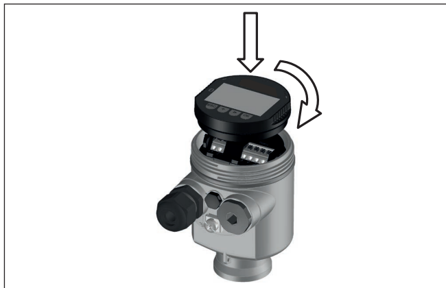
Fig. 20: Installing the display and adjustment module in the electronics compartment of the single chamber housing
