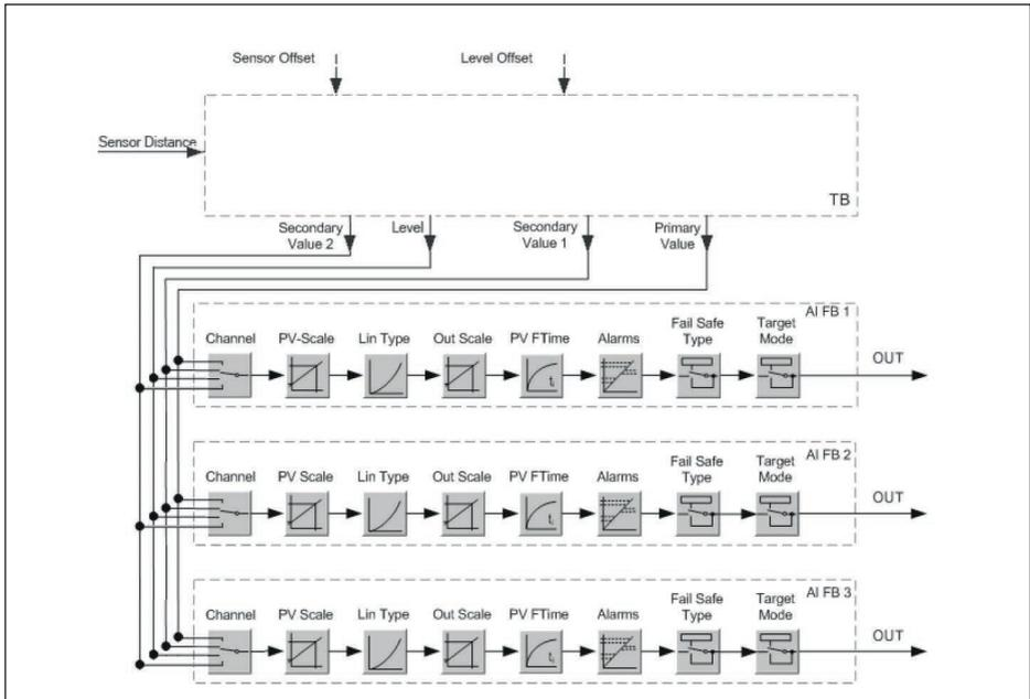
Abb. 43: VEGAFLEX 86: Block diagram with AI FB 1 ... AI FB 3 OUT values
