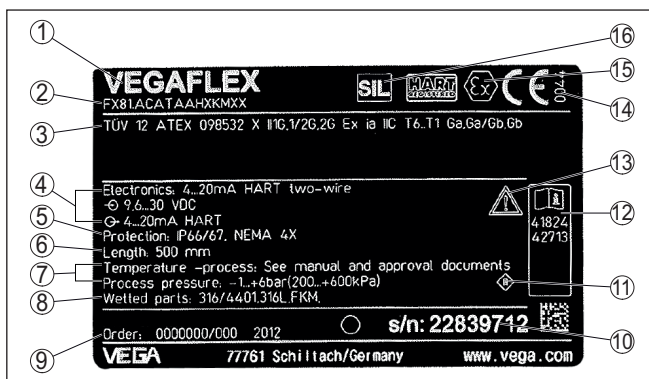
Fig. 1: Layout of the type label (example)
