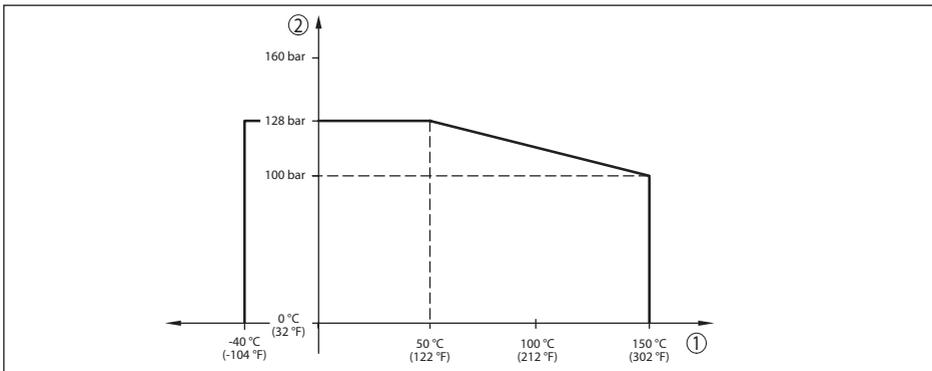
Abb. 36: Temperaturderating VEGABAR 81, Prozessanschlüsse Alloy 400 (2.4360)
