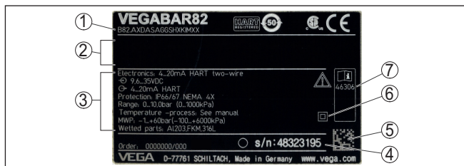
Fig. 1: Layout of the type label (example)
