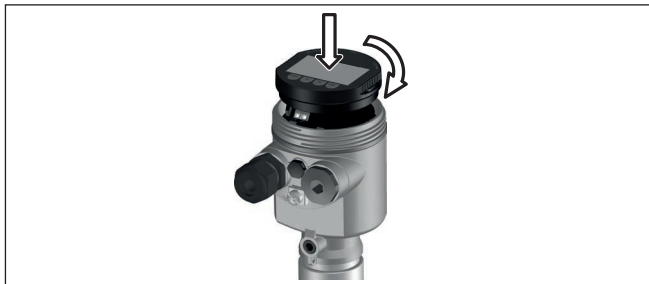
Fig. 24: Installing the display and adjustment module in the electronics compartment of the single chamber housing
