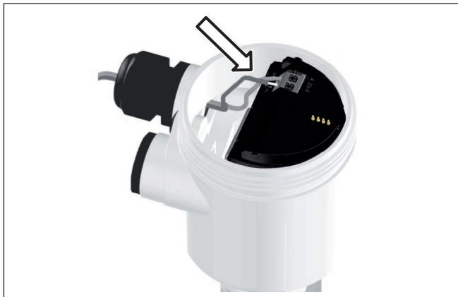
Fig. 17: Connection steps 5 and 6 - Single chamber housing
