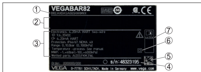
Fig. 1: Layout of the type label (example)
