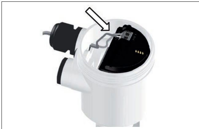
Fig. 20: Connection steps 5 and 6 - Single chamber housing
