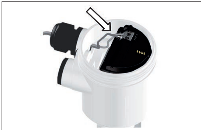
Fig. 17: Connection steps 5 and 6 - Single chamber housing
