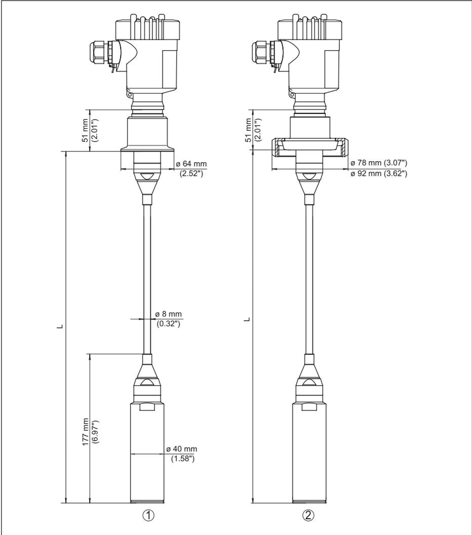
Abb. 49: VEGABAR 87, Hygieneanschlüsse
