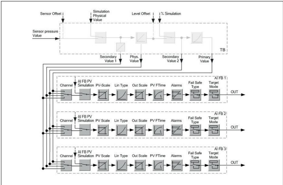
Abb. 33: VEGABAR 87: Block diagram with AI FB 1 ... AI FB 3 OUT values
