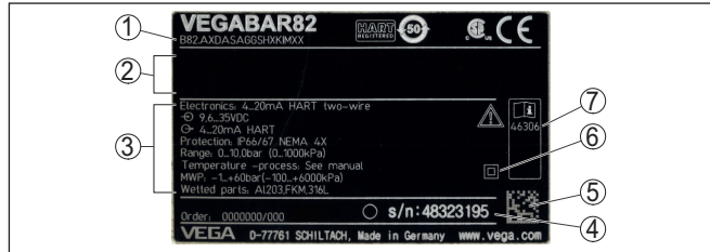
Fig. 1: Layout of the type label (example)
