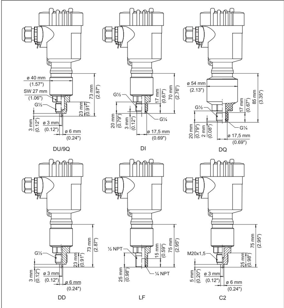
Fig. 38: VEGABAR 82, racor roscado no frontal rasante
