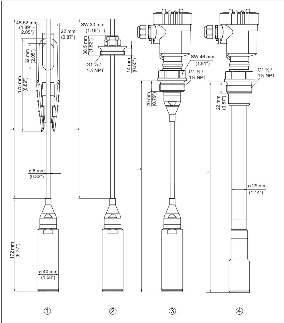
Abb. 29: VEGABAR 87, Standardanschlüsse
