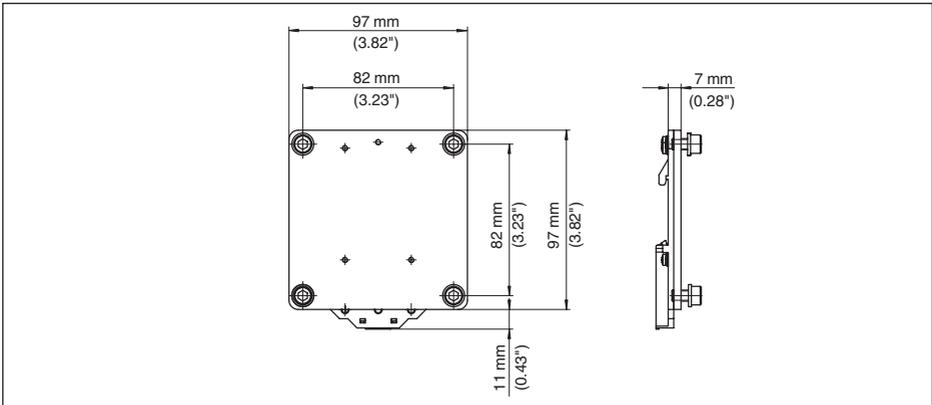
*Fig. 31: Adapter plate for carrier rail mounting of VEGADIS 82*
