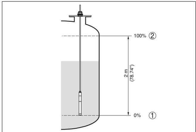
Fig. 21: Parameter adjustment example Min./max. adjustment, level measurement
