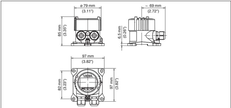
Fig. 27: VEGADIS 82 with plastic housing
