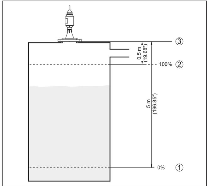
Fig. 20: Parameterisation example, Min./max. adjustment
