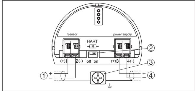
Fig. 9: Wiring plan VEGADIS 82 4 ... 20 mA/HART
