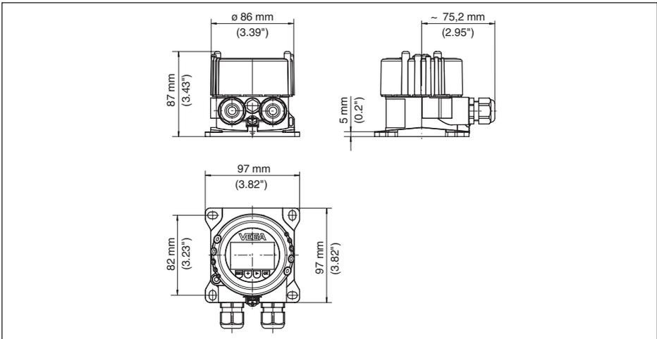
Fig. 29: VEGADIS 82 with Aluminium housing
