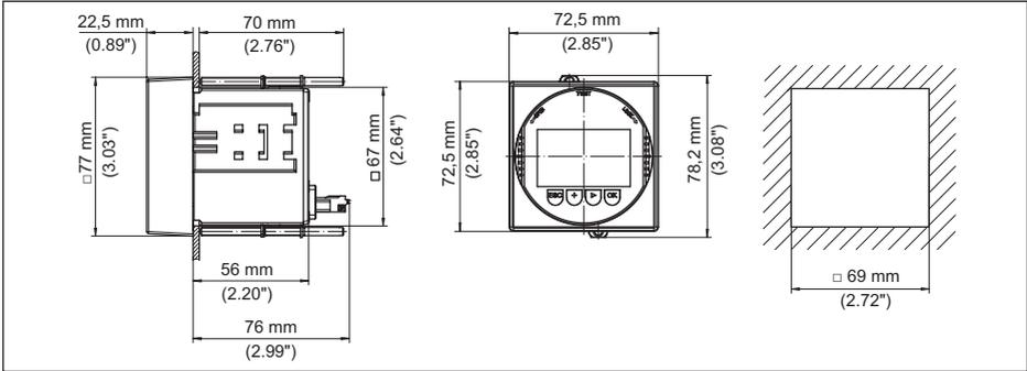
Fig. 28: VEGADIS 82 with plastic housing for panel mounting
