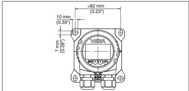
Fig. 3: Drilling dimensions for VEGADIS 82 for wall mounting
