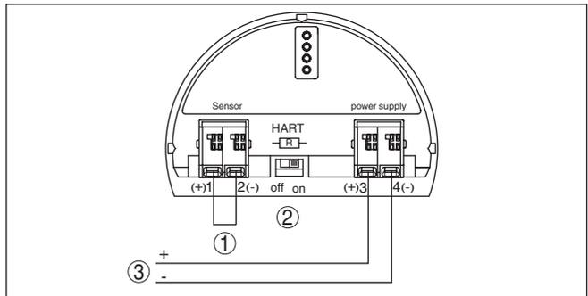
Fig. 14: Bridge between terminals 1 and 2 on the VEGADIS 82
