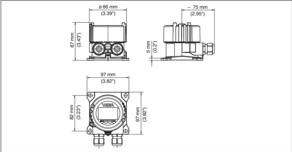
*Fig. 30: VEGADIS 82, with stainless steel housing (precision casting)*
