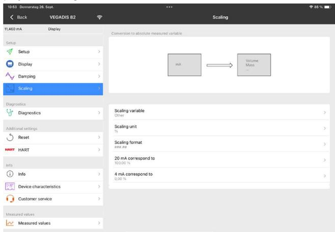
Fig. 23: Example of an app view - Setup scaling
