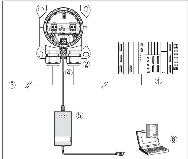
Fig. 25: Connecting the PC via HART to the signal cable
