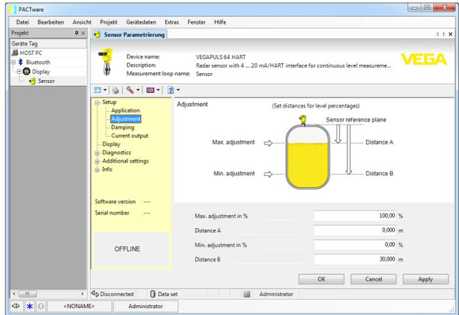
Fig. 26: Example of a DTM view
