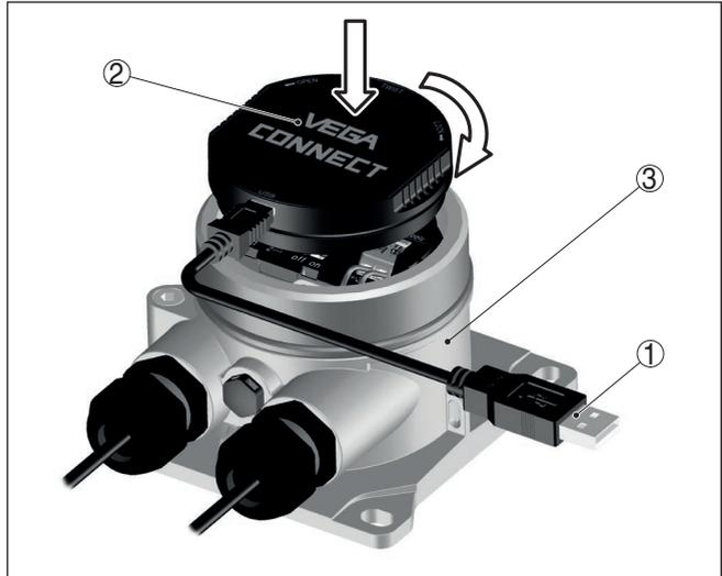
Fig. 24: Connection of the PC via interface adapter
