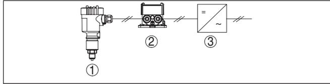
Fig. 11: VEGADIS 82 in conjunction with an individual sensor
