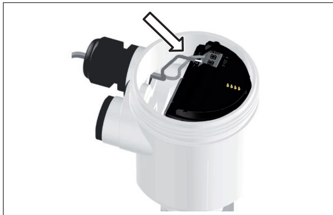
Fig. 11: Connection steps 5 and 6 - Single chamber housing
