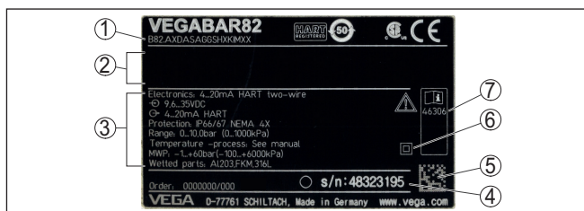
Fig. 1: Layout of the type label (example)
