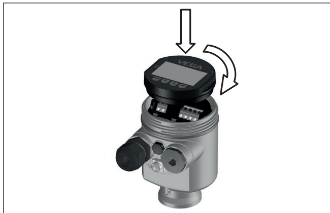
Fig. 7: Installing the display and adjustment module in the electronics compartment of the single chamber housing
