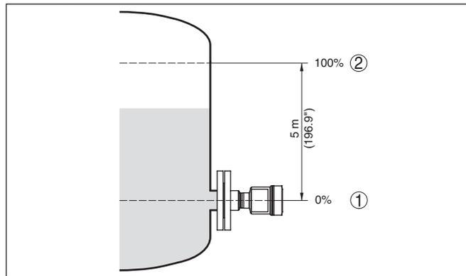
Fig. 6: Parameter adjustment example Min./max. adjustment, level measurement
