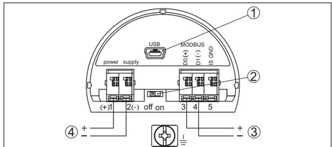
Fig. 4: Connection compartment
