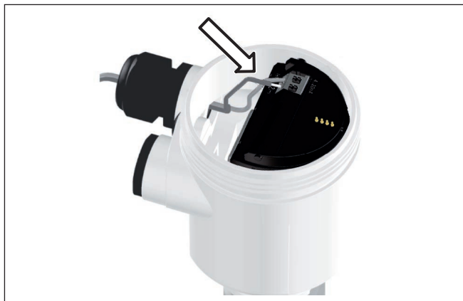
Fig. 3: Connection steps 5 and 6 - Single chamber housing
