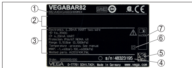
Fig. 1: Layout of the type label (example)
