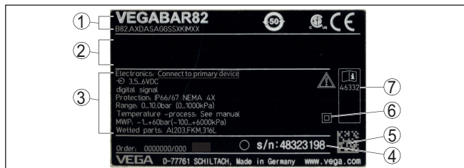
Fig. 1: Layout of the type label (example)
