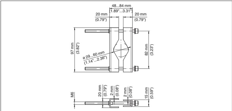
Fig. 25: Brackets for tube mounting of VEGADIS 82
