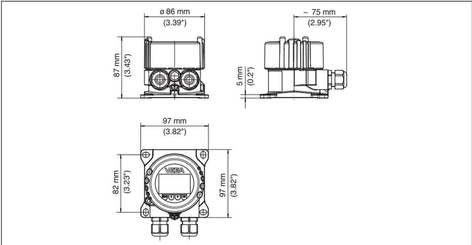
*Fig. 23: VEGADIS 82, with stainless steel housing (precision casting)*
