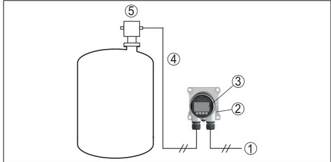
Fig. 2: Connection of VEGADIS 82 to the sensor
