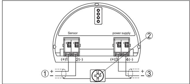
Fig. 9: Wiring plan VEGADIS 82 for 4 ... 20 mA sensors
