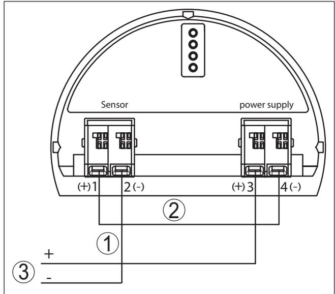
Fig. 13: Connection of VEGADIS 82 as external display to a four-wire sensor with active 4 ... 20 mA output
