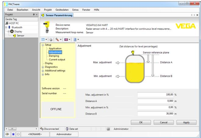
Fig. 19: Example of a DTM view
