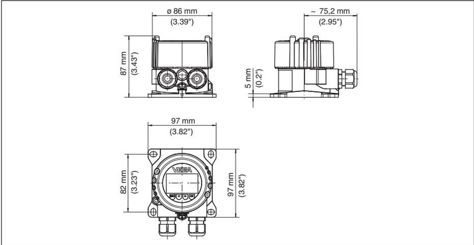
*Fig. 22: VEGADIS 82 with Aluminium housing*
