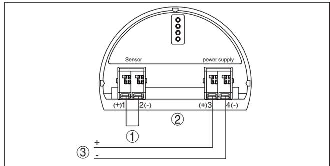
Fig. 12: Bridge on terminals 1 and 2 on the VEGADIS 82
