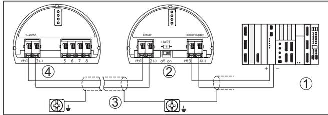
Fig. 15: Connection example 4 ... 20 mA sensor and processing system/PLC
