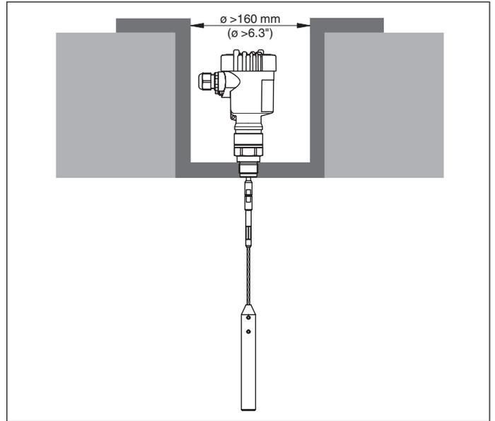
Fig. 11: Installation in concrete silo
