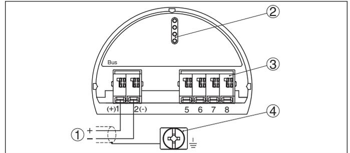
Fig. 31: Terminal compartment, double chamber housing
