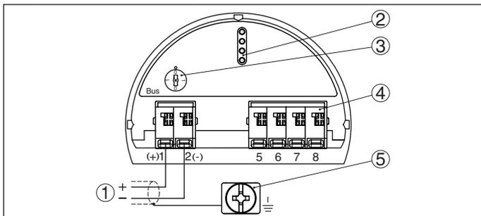
Fig. 30: Electronics and terminal compartment, single chamber housing
