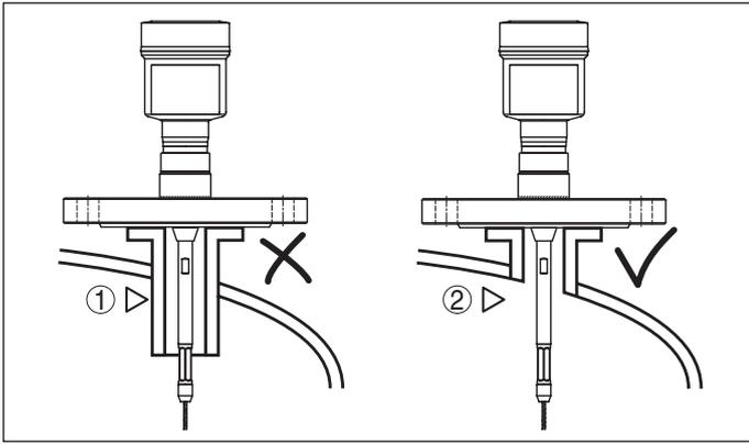
Fig. 9: Socket must be installed flush
