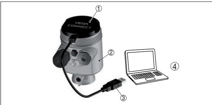
Fig. 36: Connection of the PC via VEGACONNECT and USB
