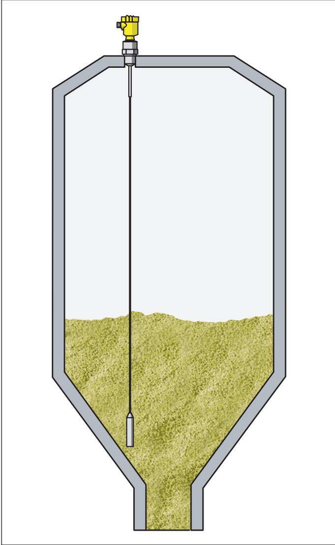
Fig. 21: Level measurement in a storage vessel with VEGAFLEX 82
