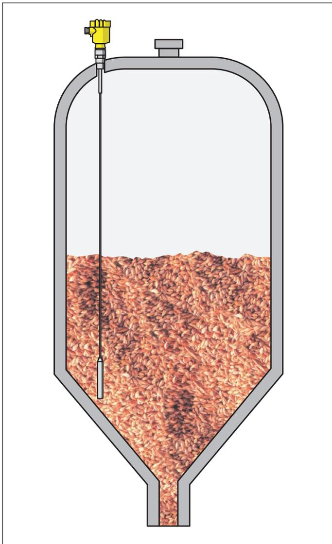
Fig. 19: Level measurement in a grain silo with VEGAFLEX 82
