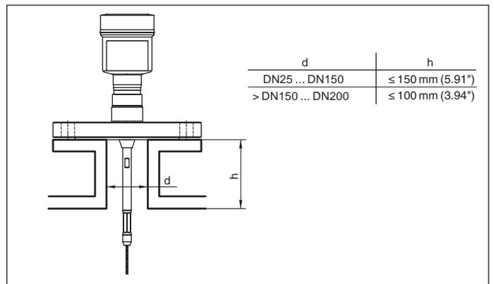
Fig. 8: Mounting socket
