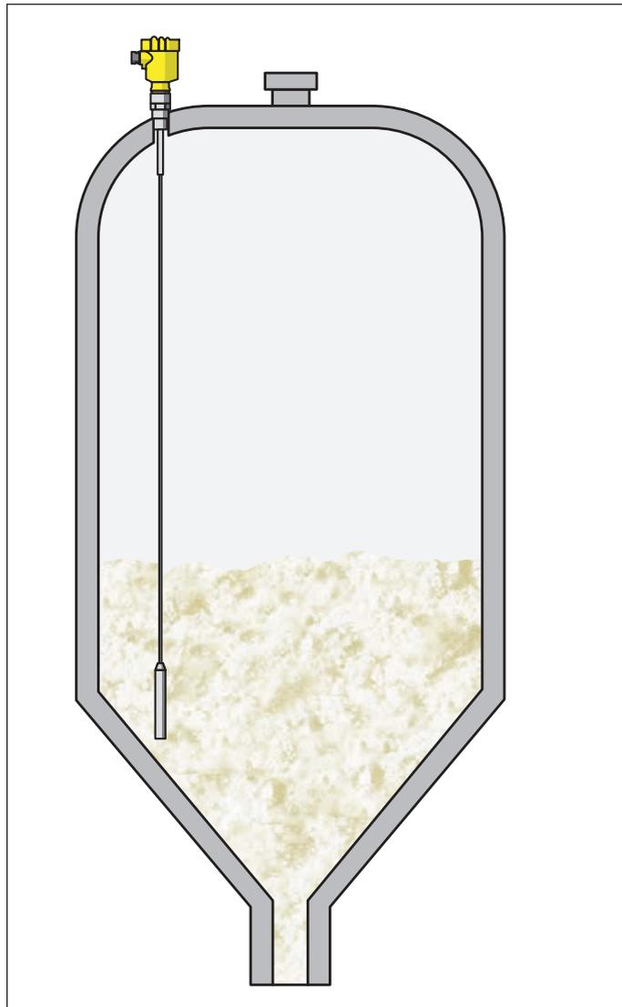
Fig. 20: Level measurement of plastic granules with VEGAFLEX 82
