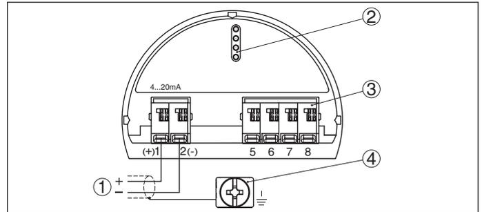
Fig. 23: Electronics and terminal compartment, single chamber housing
