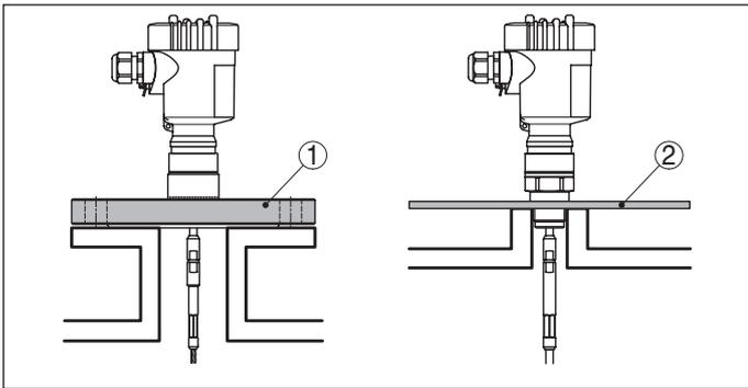
Fig. 10: Installation in plastic silo
