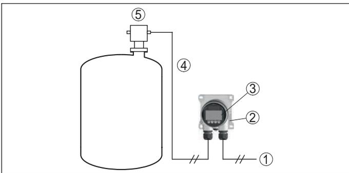
Fig. 40: Connection of VEGADIS 82 to the sensor
