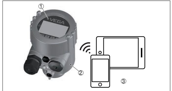
Fig. 37: Wireless connection to smartphones/tables
