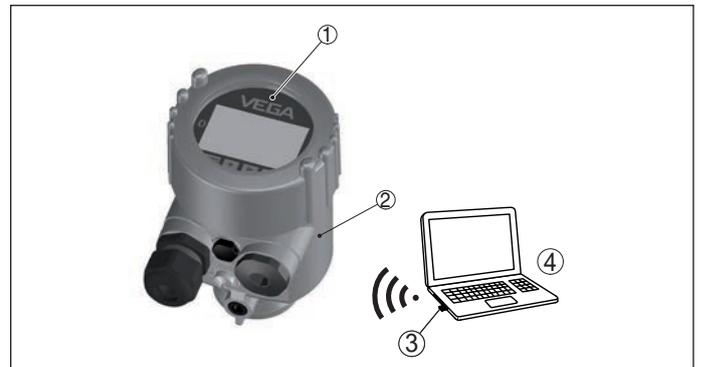
Fig. 38: Connection of the PC via Bluetooth adapter
