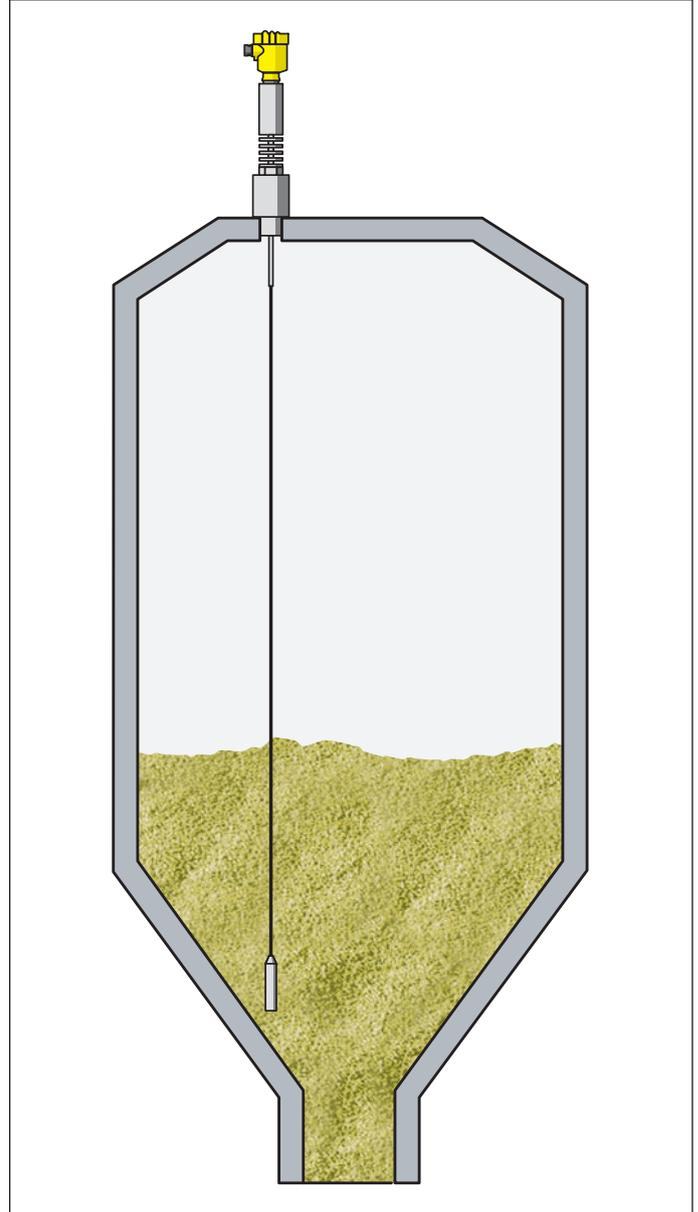
Fig. 22: Level measurement in a clinker vessel with VEGAFLEX 86
