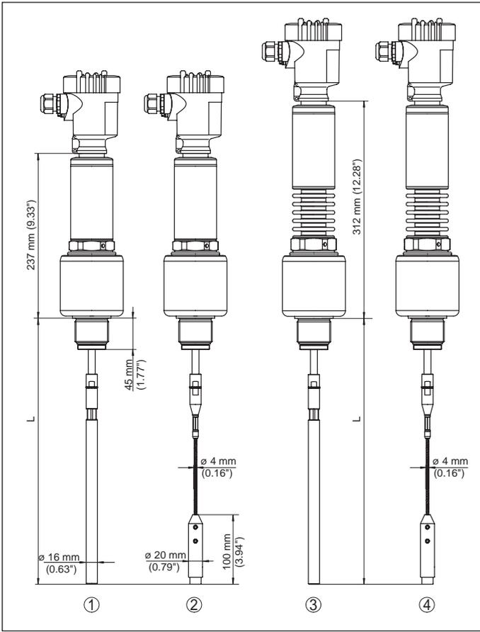
Fig. 47: VEGAFLEX 86, cable and rod version with threaded fitting
