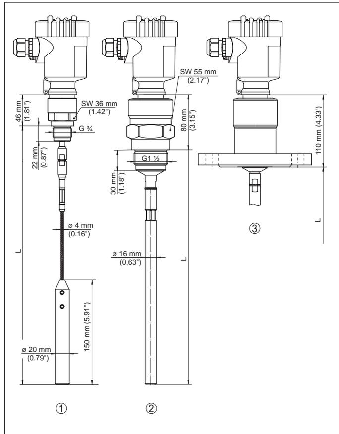
Fig. 46: VEGAFLEX 82, cable and rod version
