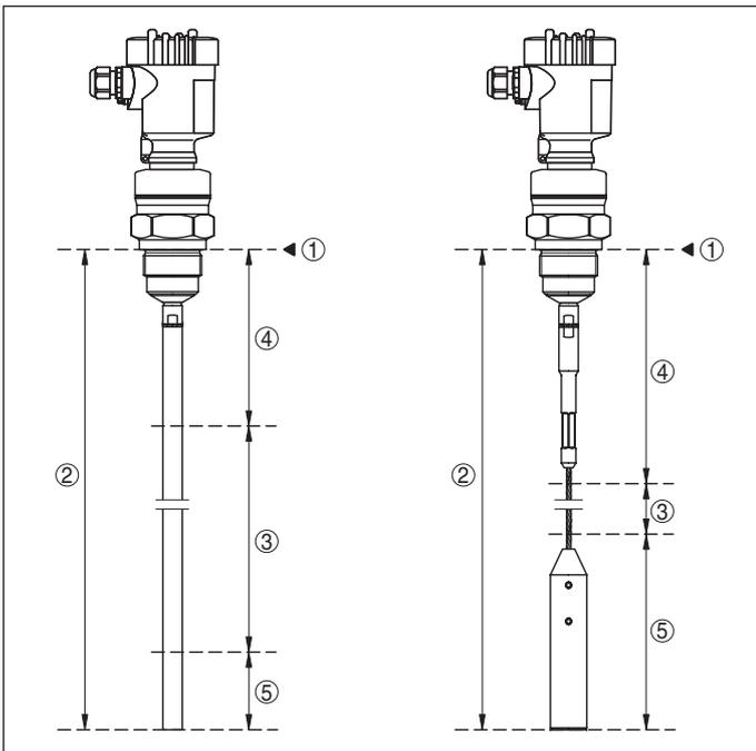
Fig. 1: Measuring ranges of VEGAFLEX
