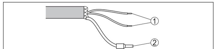
Fig. 25: Wire assignment in permanently connected connection cable
