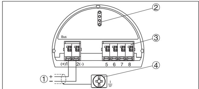
Fig. 8: Connection compartment - double chamber housing
