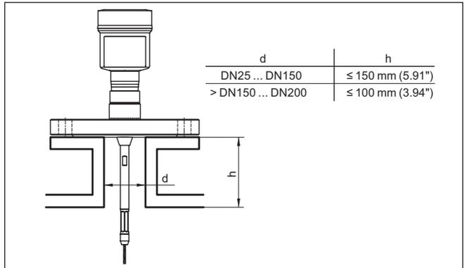
Fig. 4: Mounting socket
