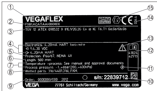
Fig. 1: Layout of the type label (example)
