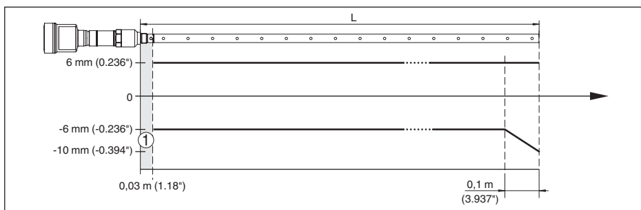
Fig. 29: Deviation VEGAFLEX 86 in coax version in water (measurement length up to 6 m/19.69 ft)
