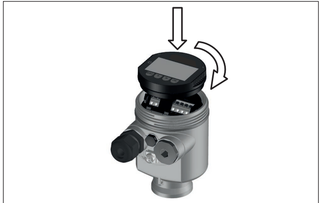
Fig. 24: Installing the display and adjustment module in the electronics compartment of the single chamber housing
