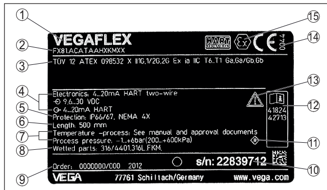
Fig. 1: Layout of the type label (example)
