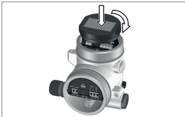
Fig. 9: Insertion of the display and adjustment module
