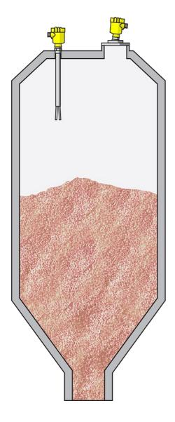
Level measurement and point level detection
