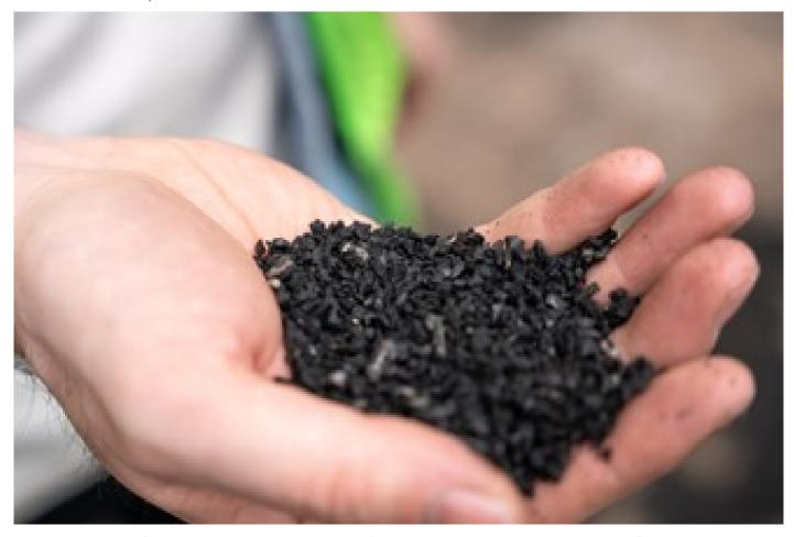
. Around 7,500 tonnes of used tyres are turned into 5,000 tonnes of rubber granulate – this is the amount that each of the two reactors converts each year.
