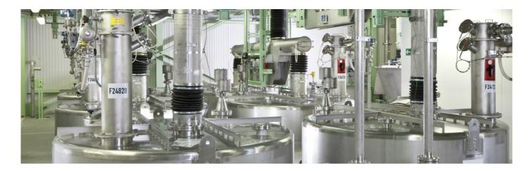
Radar level sensors ensure optimal flow in slurry and UF tanks
