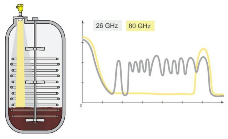
The very good signal focusing of the 80-GHz sensor enables reliable measurement of the liquid level, even in vessels with many internal installations.
