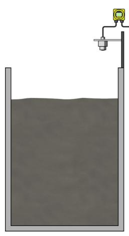
Measuring task Level measurement Measuring point Container Measuring range up to 0 ... 15 m Medium Sludge Process temperature 0 ... +30 °C Process pressure 0 ... 0 bar Special challenges Steam, condensate, buildup
