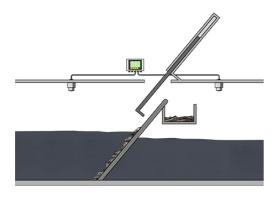
Water level measurement Measuring point Screen Measuring range up to 0 ... 5 m Medium Water Process temperature +10 ... +30 °C Process pressure 0 ... 0 bar Special challenges Buildup, abrasion, foam
