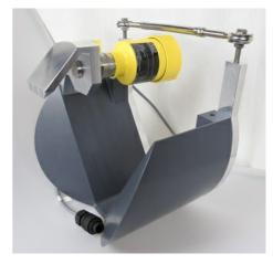
The UMS channel is available for different diameters. The conception and development of the channel was only possible thanks to the very compact design of the VEGAPULS 64 sensor
