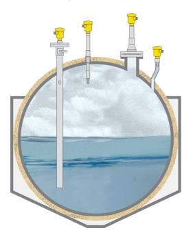
Measuring task Level and pressure measurement, point level detection Measuring point Tank Measuring range up to 40 m Medium Liquefied gas Process temperature -20 ... -162 °C Process pressure 0 ... +5 bar Special challenges Extremely low temperatures, low dielectric constants, low density, different products, ship approvals, Ex zone
