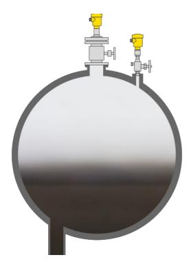
Level and pressure measurement Measuring point Sphere Measuring range up to 20 m Medium LPG Process temperature -10 ... +45 °C Process pressure +1 ... +3 bar Special challenges Low temperature, low dielectric constants
