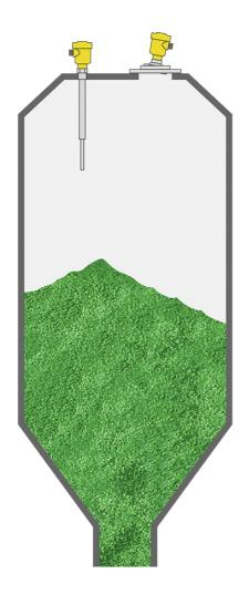
Level measurement and point level detection
