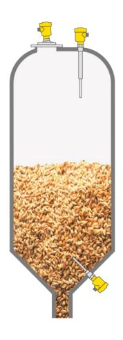
Level measurement and point level detection
