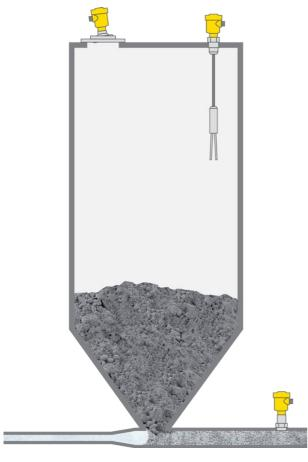
Level and pressure measurement, point level detection
