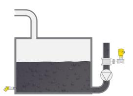
Measuring task Level and flow measurement Measuring point Tank Measuring range up to 2 m Medium Machine oil Process temperature +20 ... +80 °C Process pressure +5 ... +6 bar Special challenges High pressures
