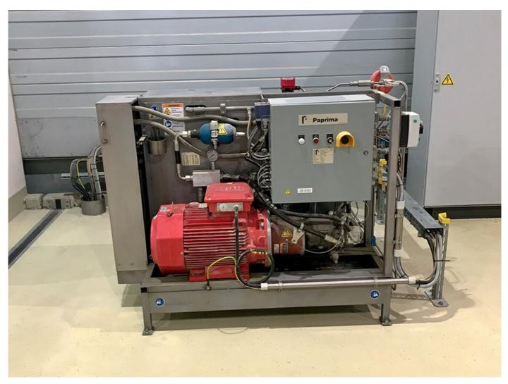
The level of the lubricating oil for the rotary lobe pumps is critical for their operation. Thanks to VEGAPULS 64, this level is now reliably monitored.
