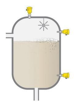
Level measurement and point level detection
