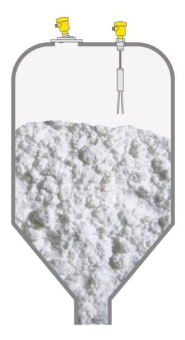
Level measurement and point level detection
