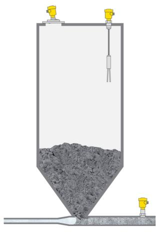
Level and pressure measurement, point level detection
